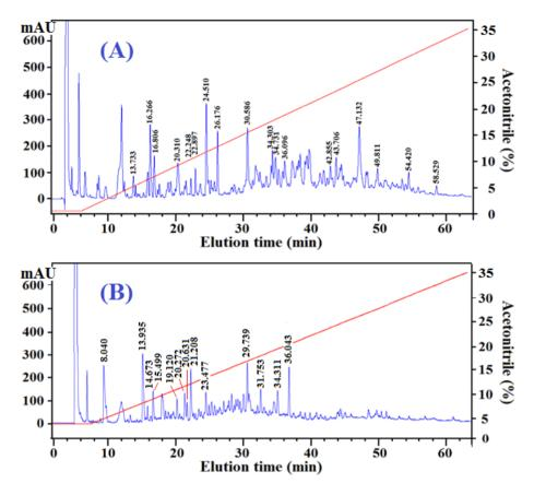
**Figure 3.** Elution profiles of Fr.A3 (**A**) and Fr.B2 (**B**) obtained by RP-HPLC on a Zorbax SB-C18 column ( $4.6 \text{ mm} \times 250 \text{ mm}$ , Agilent, USA). Absorbance was measured at 220 nm.
