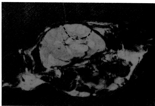
Fig. 1. Area bounded by the dashed line represents the limits of the surface coil sensitive volume(radius=9.5mm) from which the magnetic resonance spectroscopy signals arise.
