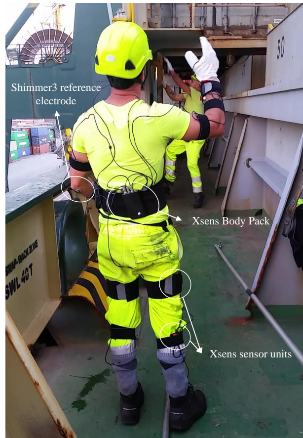
Figure 10. A volunteer ready to start his work shift wearing the wearable devices. The sensor units have been placed on the body segments as described in Section 3.4.1.
