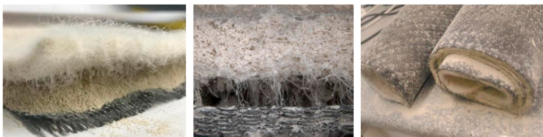
Figure 1. Geosynthetic clay liner product used in this study.
