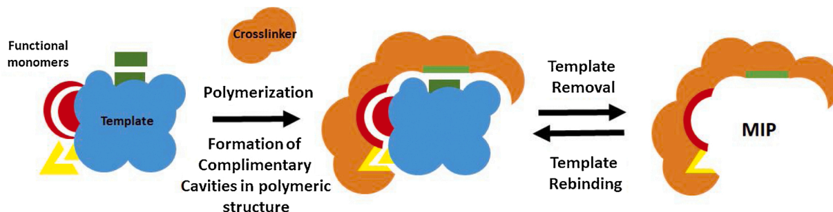
Fig. 1. A generic schematic demonstrating the fundamental principles behind the synthesis and extraction of a MIP.
