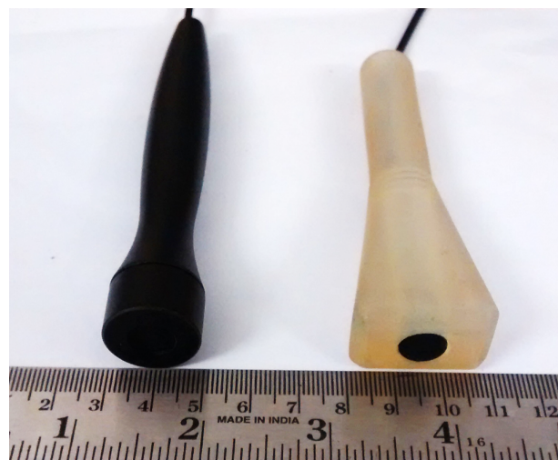
FIGURE 4. Single element ultrasound probes designed for ARTSENS.
