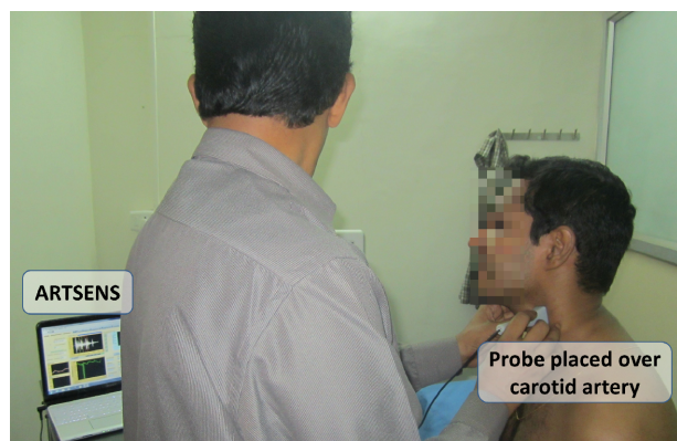
FIGURE 3. ARTSENS used to perform carotid artery stiffness measurement of a volunteer.
