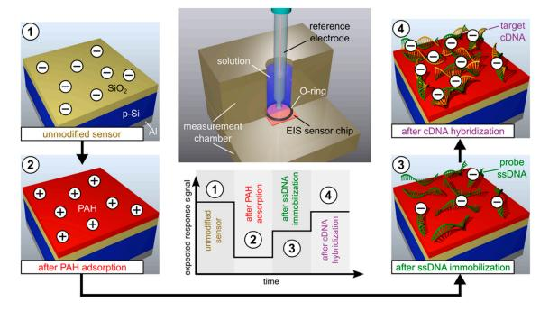
**Figure 5.** Modification steps of the EIS sensor, measurement setup (middle column, top), and expected ConCap response (middle column, bottom). (1) Unmodified sensor, (2) after poly(allylamine hydrochloride) (PAH) adsorption, (3) after single-stranded DNA (ssDNA) immobilization, and (4) after complementary target DNA (cDNA) hybridization. + and – symbols indicate the respective surface charges. Reproduced from Ref. [144] with permission of the American Chemical Society.
