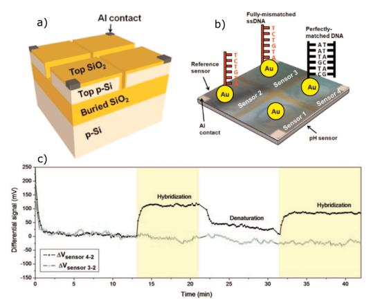
**Figure 8.** Schematic of the bare (a) and AuNP-modified (5–8 nm) (b) EIS chips combining four individually addressable EIS sensors prepared using a silicon-on-insulator wafer and a differential-mode ConCap response after consecutive DNA hybridization, denaturation, and rehybridization (c).  $\Delta V_{4-2}$  and  $\Delta V_{3-2}$ : net differential signals between sensor 4 and sensor 2 and sensor 3 and sensor 2, respectively. Adapted from Ref. [135] with permission from Wiley-VCH.
