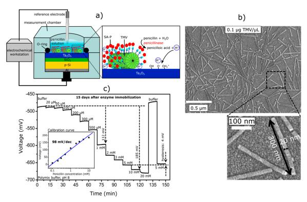
**Figure 4.** Schematic structure of an enzyme-modified capacitive EIS (EnEIS) biosensor modified with *tobacco mosaic virus* (TMV) particles as enzyme nanocarriers (**a**), scanning electron microscopy image of TMV particles on the  $Ta_2O_5$  surface (**b**), and the sensor signal in buffer solution with different penicillin concentrations (**c**). Adapted from Ref. [103] with permission of Elsevier.
