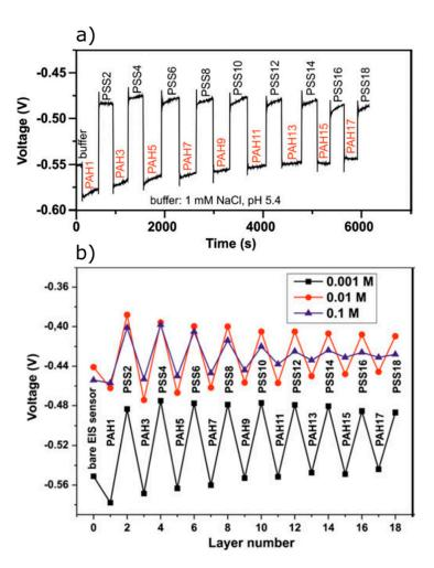
**Figure 6.** Electrical monitoring of the PE multilayer build-up with a p-Si–SiO $_2$  EIS sensor. (a) ConCap response and (b) potential shifts as a function of the PE layer number and ion concentration. The PAH and poly(sodium 4-styrenesulfonate) (PSS) layers were deposited from a 50  $\mu$ M PE solution adjusted with different NaCl concentrations of 100, 10, and 1 mM (pH 5.4). Reproduced from Ref. [172] with permission from Springer.
