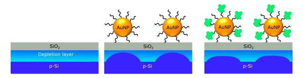
**Figure 7.** Schematic of a AuNP-modified capacitive EIS sensor. Expected modulation of the depletion layer after the deposition of negatively charged citrate-capped AuNPs and after the binding of positively charged molecules on AuNPs are exemplarily shown for a p-type EIS structure.
