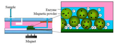
**Figure 3.** Operating principle of a microfluidic chip. Enzyme-carrying alginate microbeads are immobilized on the EIS-sensor surface by means of an external magnetic field. The sample is injected into the microchannel and reacts with the enzyme contained in alginate beads. The change in potential on the sensor surface induced by the release of hydrogen ions during the reaction process is measured. Reproduced from Ref. [82] with permission of Elsevier.
