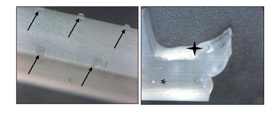
**Figure 5.** Images of the fabricated resin material taken with a digital microscope. (a) Intact test specimen, surface on the edge. The black arrows point to the protrusions, which are the remains of the raft. (b) Broken test specimen. The black star indicates the broken, the asterisk marks the intact surface, where the glassy-like structure can be observed. Magnification:  $35 \times$ .
