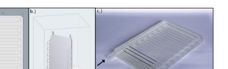
**Figure 2.** (a) The CAD model of the cooling plate created with Rhinoceros 6 CAD software. (b) The .stl model uploaded in the slicer software. (c) The manufactured cooling plate using a 3D printer. The arrows indicate the inflow and outflow pipes of the plate, and the dotted lines represent the parallel cooling pipes.
