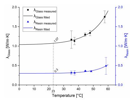
**Figure 3.** Measured and fitted heat conduction parameters of the tested materials. Heat conduction of the reference glass material is represented by the black curve; the squares show the average values with standard deviations measured at the indicated temperatures. Heat conduction parameters of the resin material are represented by the blue curve; triangles show the measured average values with standard deviations measured at the indicated temperatures.
