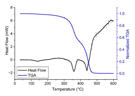
**Figure 4.** Heating curves of clear resin V4 (30–600 °C, black line) combined with TGA of the samples (30–600 °C, blue line) on a common temperature scale (i.e., abscissa) at a heating rate of 10 °C/min. On the heating curves, the endothermic process (i.e., when the sample melts) causes a drop in heat flow. A decrease in normalized TGA indicates loss of sample mass. The error bars show the standard error of means from at least 3 independent measurements.
