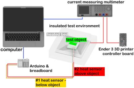
Figure 1. Schematic representation of the experimental setup used for thermal conductivity measurements.
