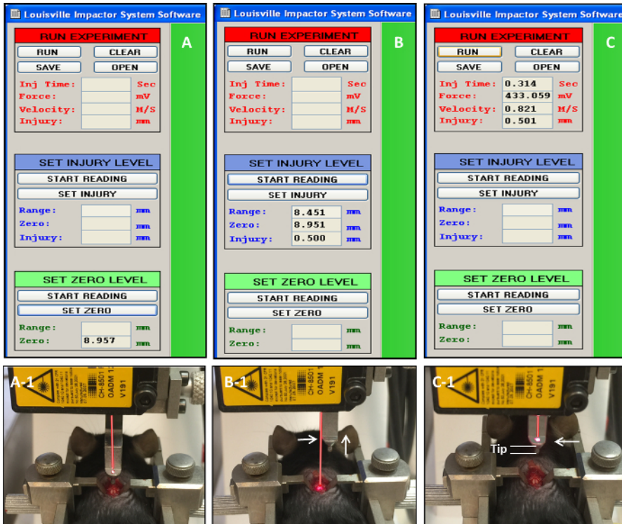
Figure 3: Method to Produce a Contusive SCI. (A-C) The Graphical User Interface (GUI) software with three injury parameters/zones are shown. (A, A-1) The green zone (SET ZERO LEVEL) calibrates the distance of the plunger tip. The red line indicates the laser beam path. (B, B-1) The blue zone is used to set the injury level (SET INJURY LEVEL). The impactor is lifted up and moved laterally to the right side to allow the laser beam to reach the dorsal surface of the spinal cord to set the zero level. The red line indicates the laser beam path. (C, C-1) Prior to impact, the tip is moved back onto the laser beam path to execute the injury (RUN). The injury parameters are under the red zone (RUN EXPERIMENT). The red line indicates the laser beam path. Please click here to view a larger version of this figure.
