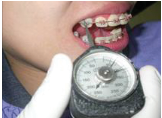
Figure 2: Recording the amount of stretching force with a Correx gauge
