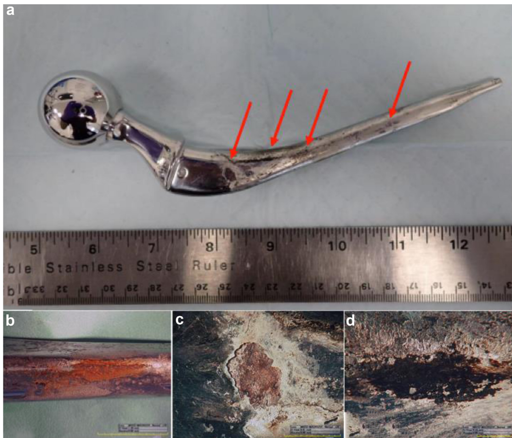
Figure 3. (a) An explanted stem with corrosion pits highlighted with arrows, (b) red-colored corrosion residue with high levels of iron, (c) a large corrosion pit with white-colored corrosion residue, and (d) a corrosion pit over 1.5mm deep with black-colored corrosion residue.
