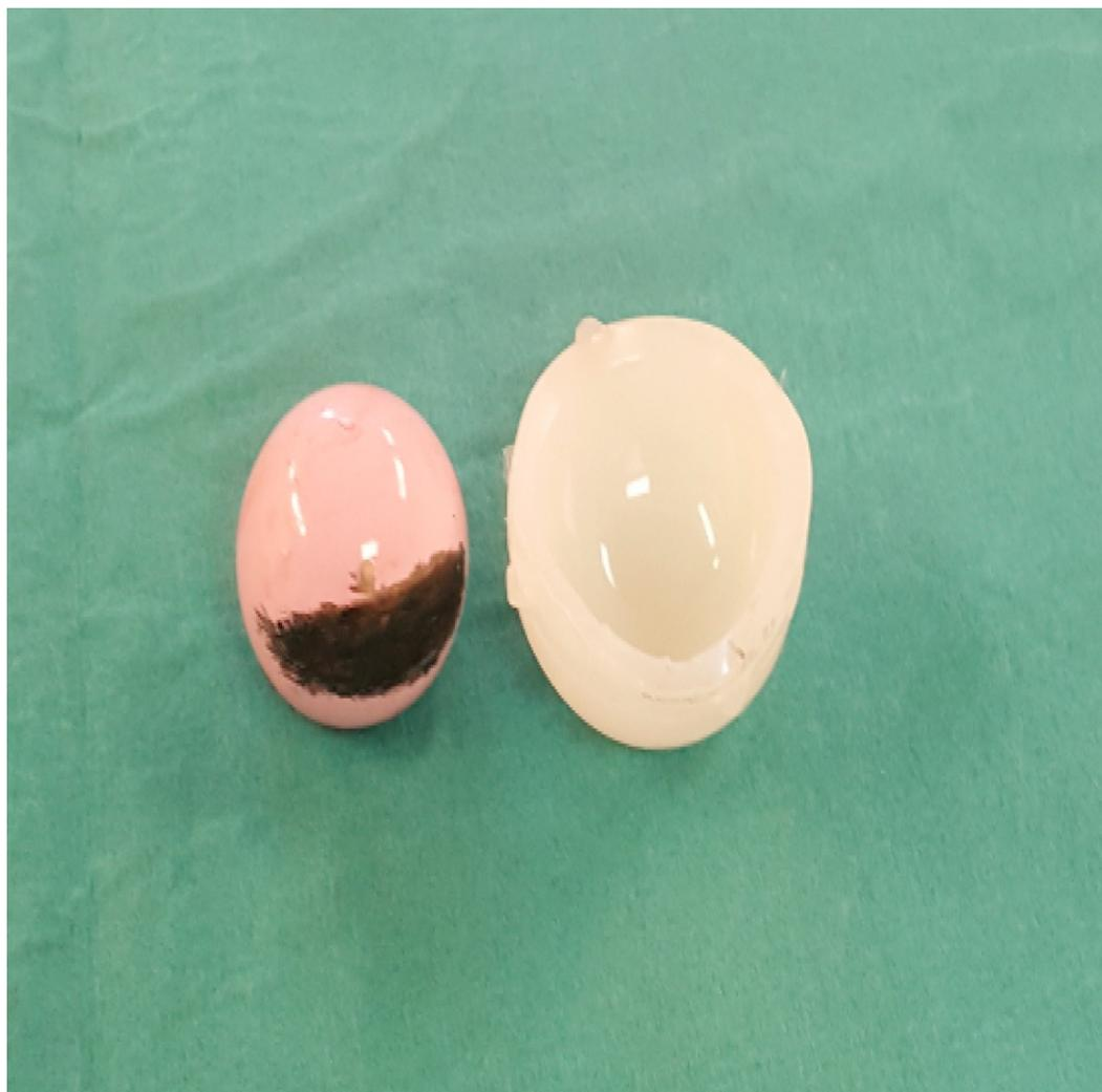
**FIGURE 5: Explanted acetabular cup with marked stripe wear seen as dark discolouration of pink ceramic head and deformed explanted acetabular liner**
