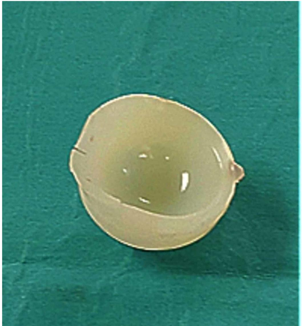
**FIGURE 6: Explanted dissociated polyethylene liner with marked plastic deformation of the rim, new oval shape and multiple tine loss**
