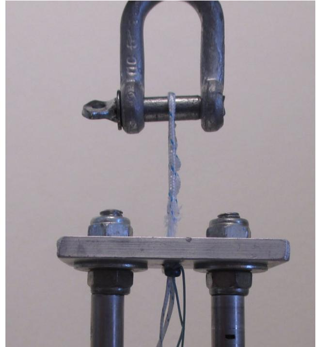
**Figure 2.** UltraButton in the isolated device testing setup.
