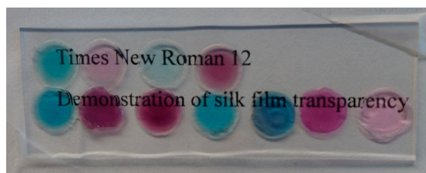
Figure 5. Photograph of selected silk–dye–patches (red for neutral red and blue for thionine) on a glass slide. Behind the patches and the glass slides are lines of text to illustrate the transparency of the patches. For convenience, the patches were wetted to adhere on the glass slide.
