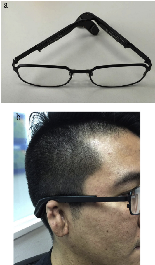
Fig. 3. a. The spectacle bone conduction hearing aid. b. A microtia patient wearing a spectacle bone conduction hearing aid.
