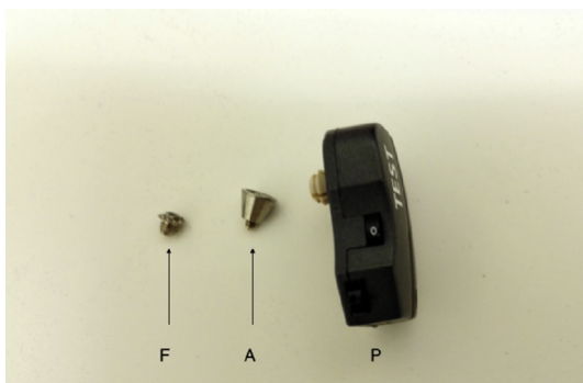
Fig. 4. Components of the percutaneous bone anchoring hearing aid system. The fixture (F), the abutment (A) and the sound processor (P).
