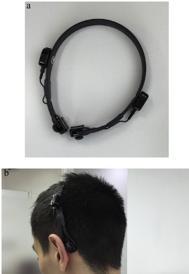
Fig. 1. a. The headband bone conduction device. b. A patient putting on a headband bone conduction device.
