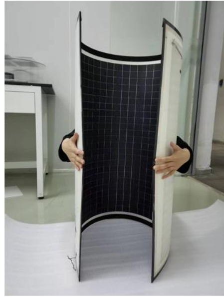
Supplementary Fig. 9 | Large module made from the flexible SHJ solar cells, featuring characteristics of light weight and rolling nature.
