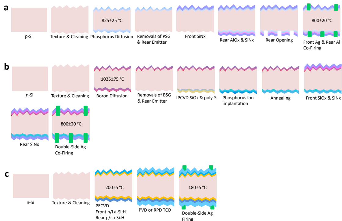
Supplementary Fig. 6 | Current fabrication of industrial c-Si solar cells. The peak temperatures of the a , PERC, b , TOPCon and c , SHJ solar cells were 825 \pm 25 \text{ }^{\circ}\text{C} , 1025 \pm 75 \text{ }^{\circ}\text{C} and 200 \pm 5 \text{ }^{\circ}\text{C} , respectively. The firing contact between TCO layers and low-temperature Ag electrodes were realized at relatively low temperatures. Large-scale flexible manufacturing was feasible for SHJ technology because of the low process temperatures and symmetrical structural design.
