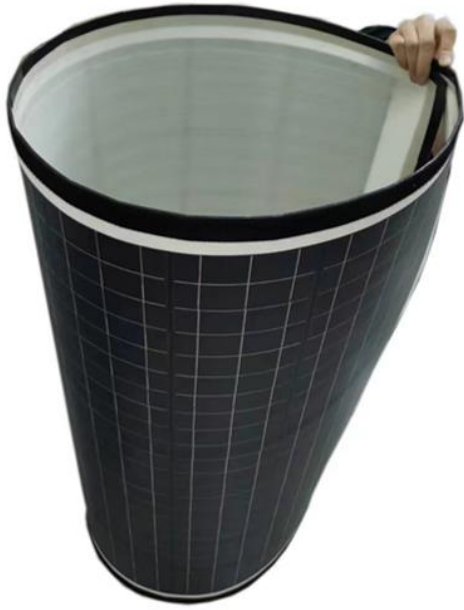
Supplementary Fig. 9 | Large module made from the flexible SHJ solar cells, featuring characteristics of light weight and rolling nature.
