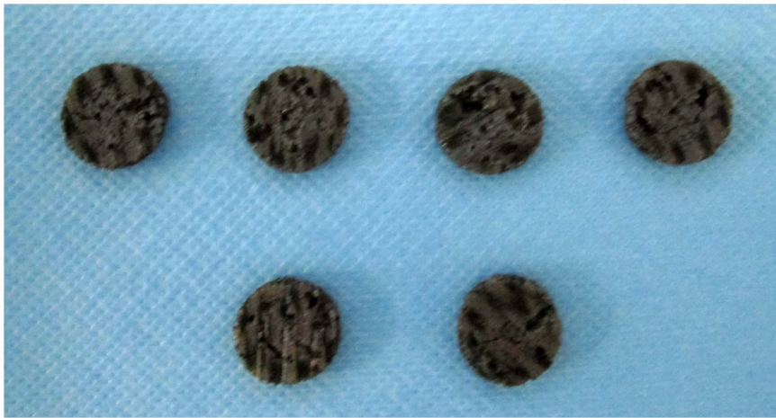
Figure 6. The titanium-niobium alloy specimens with different porosity. doi:10.1371/journal.pone.0079289.g006
