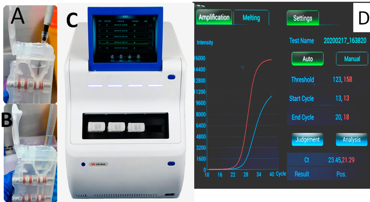
Figure 2. AIGS flow chart. A: add 10ul magnetic beads; B: add 200ul sample to each cartridge; C: Inserting the cartridge into detection site; D: result analysis. Thermal cycling conditions were as follows: reverse transcription, 56°C for 15 min; initial denaturation, 94°C for 1 min; and 40 cycles of 95°C for 10 s and 58°C for 30 s. The amplification curve was displayed on the screen in real time while the amplification programme ran.
