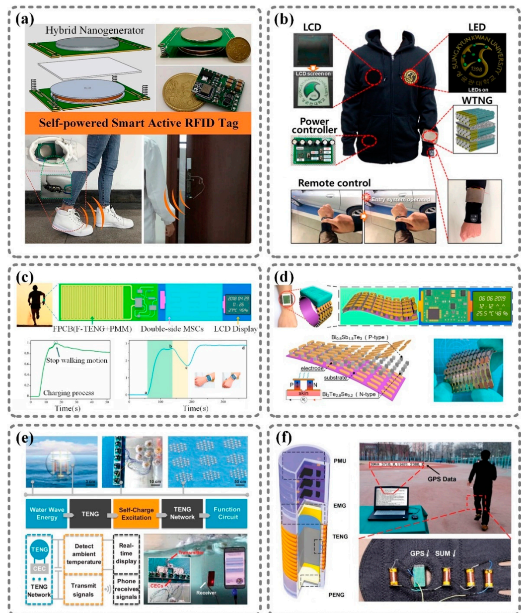
Figure 5. Self-powered systems with power management modules using nanoenergy. (a) Triboelectric-electromagnetic hybrid nanogenerator: self-powered RFID tag integrated with a hybrid nanogenerator [31]. (b) Nanopatterned textile-based wearable triboelectric nanogenerator: self-powered smart suit based on a textile-based wearable TENG [70]. (c) FPCB integrated with TENG, PMM, MSC and functional circuit: self-powered smart bracelet based on a freestanding-mode TENG [71]. (d) Thermoelectric grains bonding on flexible polyimide substrate: self-powered wearable monitoring system with a flexible thermoelectric generator (TEG) [72]. (e) TENG network with spring-assisted multilayered structure: water wave energy harvesting system that can power electronic thermometer and RF transmitter [73]. (f) Battery-like self-charging universal module for motional energy harvest: universal self-charging module composed of a “three-in-one” hybrid nanogenerator (electromagnetic generator (EMG), TENG, and piezoelectric nanogenerator (PENG)) and power management unit, which can support a GPS system. [74]. Reproduced with permission from John Wiley and Sons [73,74], Elsevier [31,71,72], and American Chemical Society [70].
