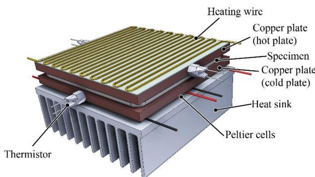
**Figure 2.** Assembly of the hot-plate measuring unit without thermal insulation.
