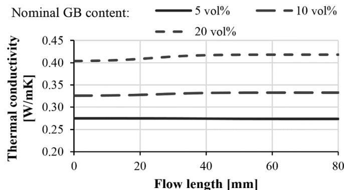
**Figure 12.** Calculated thermal conductivity of glass bead (45–75  $\mu\text{m}$ )-filled polypropylene along the flow length.
