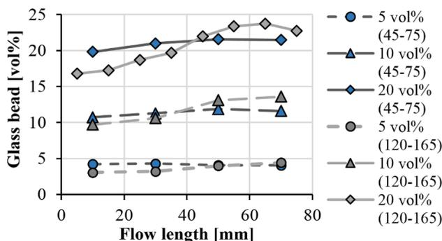
**Figure 5.** Glass bead concentration along the flow length as a function of bead size.
