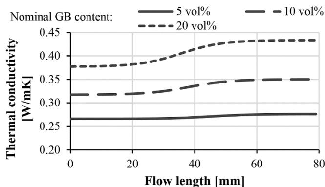
**Figure 13.** Calculated thermal conductivity of glass bead (120–165  $\mu\text{m}$ )-filled polypropylene along the flow length.
