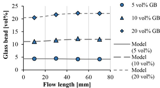
Figure 7. Segregation of the glass beads along the flow path (measurement results and the fitted model; GB size: 45–75 μm).
