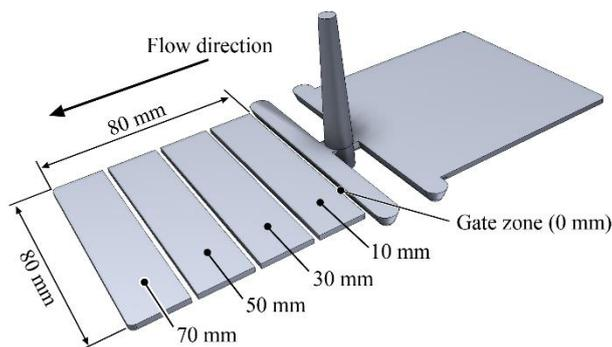
**Figure 1.** Preparation of the sample for the investigation of segregation.
