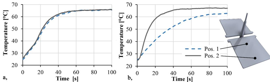
**Figure 10.** Heating curves of the injection-molded 20 vol % GB filled samples (a, GB size: 45–75 µm; b, 120–165 µm).
