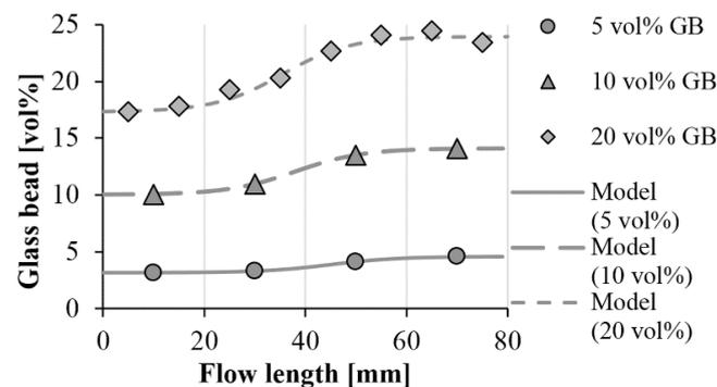
Figure 8. Segregation of the glass beads along the flow path (measurement results and fitted model; GB size: 120–165 μm).
