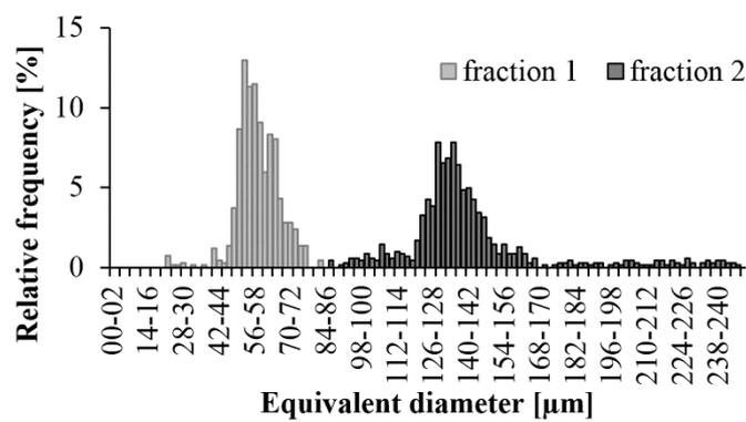
Figure 3. Glass bead size distribution after fractionating.
