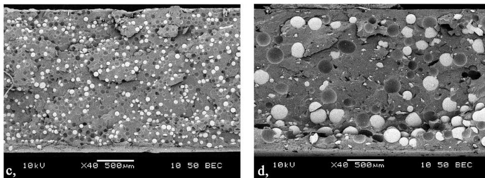
**Figure 4.** Distribution of the glass beads (20 vol %) in the injection-molded sample (45–75 μm: **a**, gate zone; **c**, end of the flow; 120–165 μm: **b**, gate zone; **d**, end of the flow).
