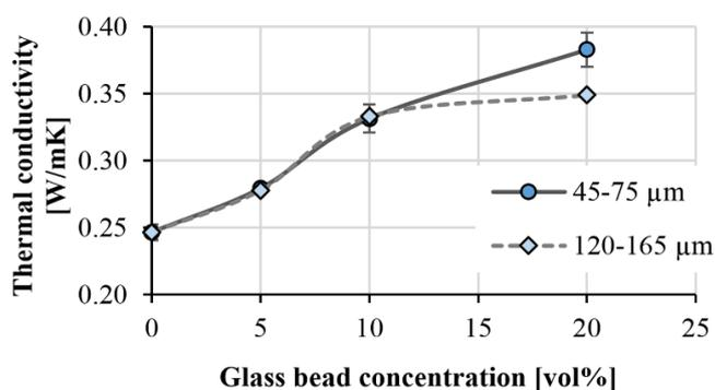
**Figure 9.** Thermal conductivity of filled polypropylenes.
