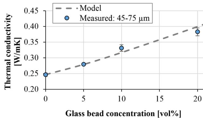
**Figure 11.** Comparison of the measured and modeled thermal conductivity (glass bead size: 45–75  $\mu\text{m}$ ).
