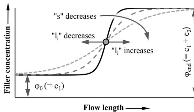
Figure 6. Interpretation of the factor of the logistic curve used to describe the segregation along the flow length.
