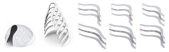
Figure 16. Form-conversion into a multi-layered sandwich shell made from developable surfaces.
