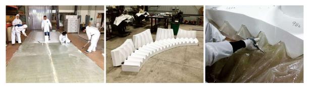
**Figure 18.** The sandwich core is made from a thin layer of glass-fiber reinforced plastic (GFRP) and pressed into form using a Styrofoam mold that was custom-made on a 4-axis hotwire machine.
