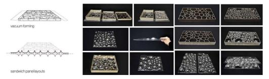
**Figure 8.** Single and double-layered PETG sandwich panels were fabricated to study the influence of different formwork parameters like materiality, height, and orientation of the mold.
