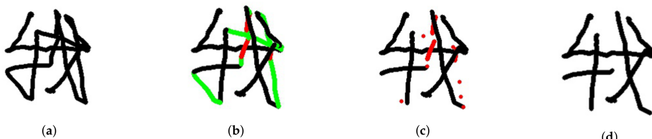
Figure 10. Steps involved in removing redundant connections from Chinese characters: (a) all trajectories appear in a single curve or stroke; (b) all redundant connections are found (the green segments represent the connections from the bottom right to the top left, while the red segments represent the connections from the bottom left to the top right with a steep slope); (c) all of the green segments are removed; and (d) the final results after the red segments are removed.
