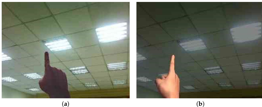
Figure 8. Challenging cases of fingertip detection in: (a) a very light environment; and (b) a very dark environment.
