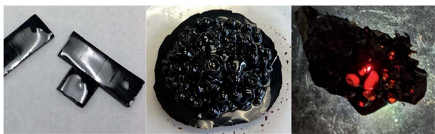
Fig. 1 Shaped materials can be fabricated from TTS_x thermosets by curing the comonomer solution at 150 °C in a mould or on a substrate, as illustrated by the rectangular prismatic brick (left) and patterned disc-shaped item (centre). A backlit sample of TTS_x (right) better illustrates the red colour and transparency of the material.
