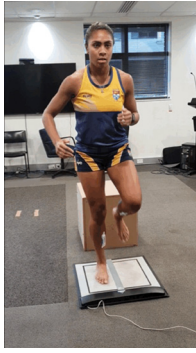
Figure 1 TekScan set up. Post-anterior cruciate ligament reconstructed athlete performing hop test, landing. Figure shows ViMove sensor placement along pretibial border and TekScan pressure plate.
