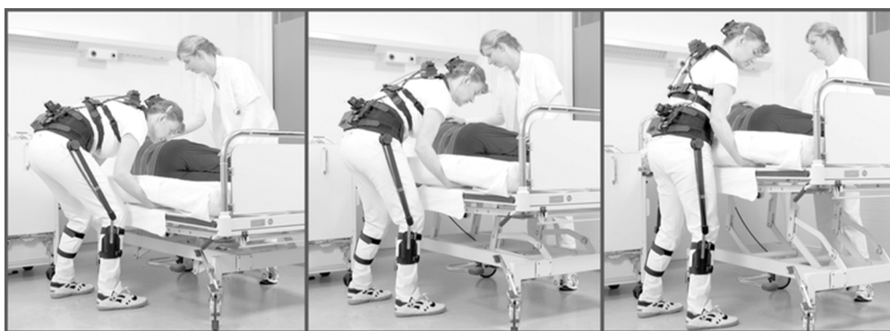
1 Standardized routine of different care activities at three different bed heights: upper edge of mattress at knee height, thigh height, and hip height.
