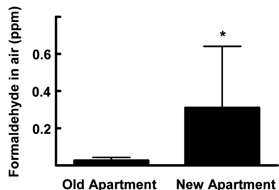
Fig. 1. Indoor formaldehyde levels in old and new apartments. Air samples were collected in the bedroom of 7 old apartments and 15 new apartments, and the concentration of formaldehyde was determined as described in Materials and methods. Values are represented as mean \pm S.D. *, P < 0.05 .
