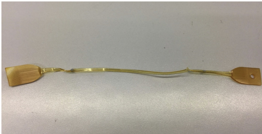
Figure 10. Dumb-bell test piece after elongation process.
