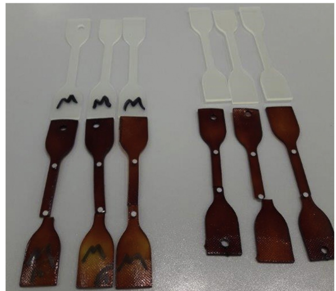
Figure 9. Difference in appearance between aged and un-aged samples.
