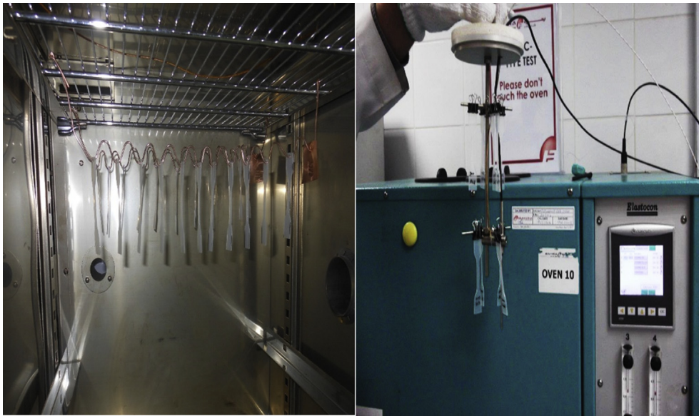
Figure 7. Insertion and suspension of dumb-bell test pieces into ageing ovens.
