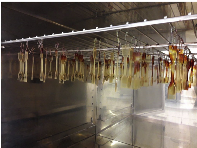
Figure 8. Dumb-bell test pieces under thermal ageing process inside drying oven.
