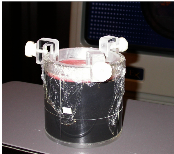
FIG. 2. The daily quality assurance phantom positioned for verification of treatment room calibration for the ultrasound image guided radiation therapy system.
