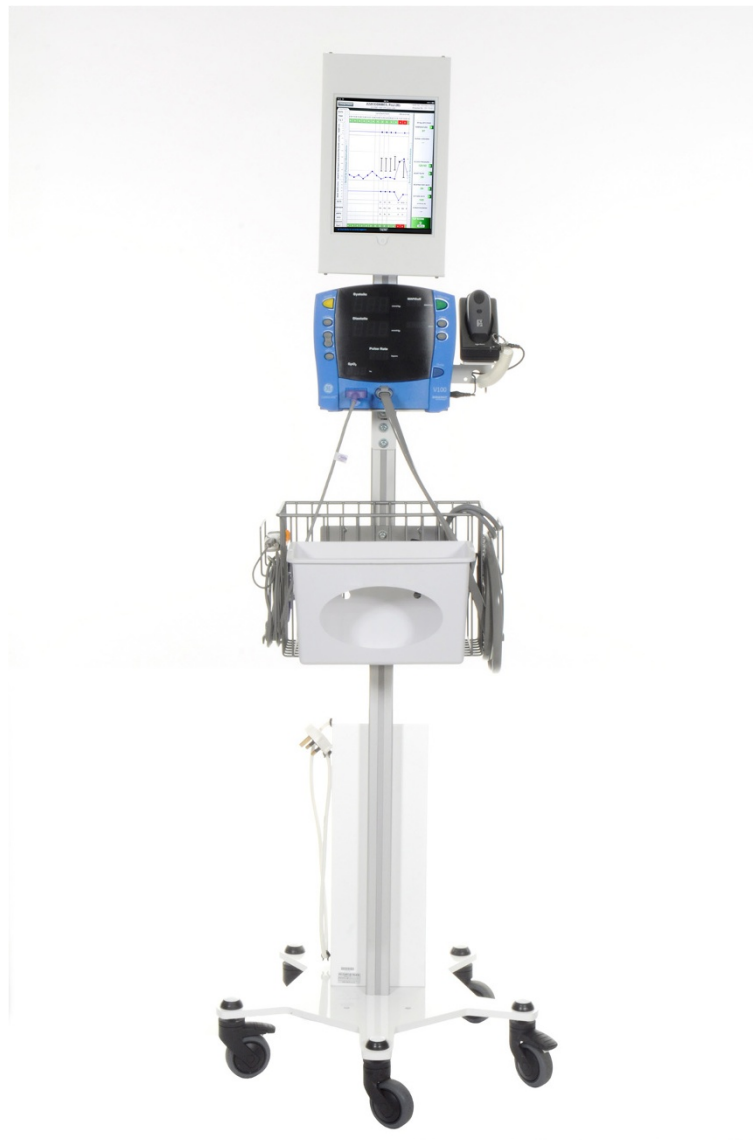
Fig. 2 The prototype SEND stand. The two novel design features of the roll stand were the mounting for the tablet computer and the provision of an enclosed power distribution board to which both the patient monitor and tablet computer power cables were connected. This enables all the system components to be charged using a single cable
