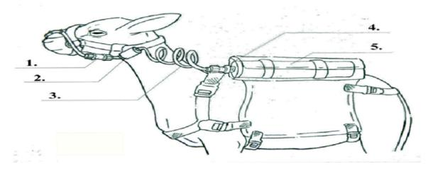
**Figure 2.** Components of the device used for measuring CH<sub>4</sub> emission. Illustration of components to collect CH<sub>4</sub>: **1.** Flow control valve; **2.** particle filter; **3.** spiral hose; **4.** quick connect; **5.** stainless cylinder.
