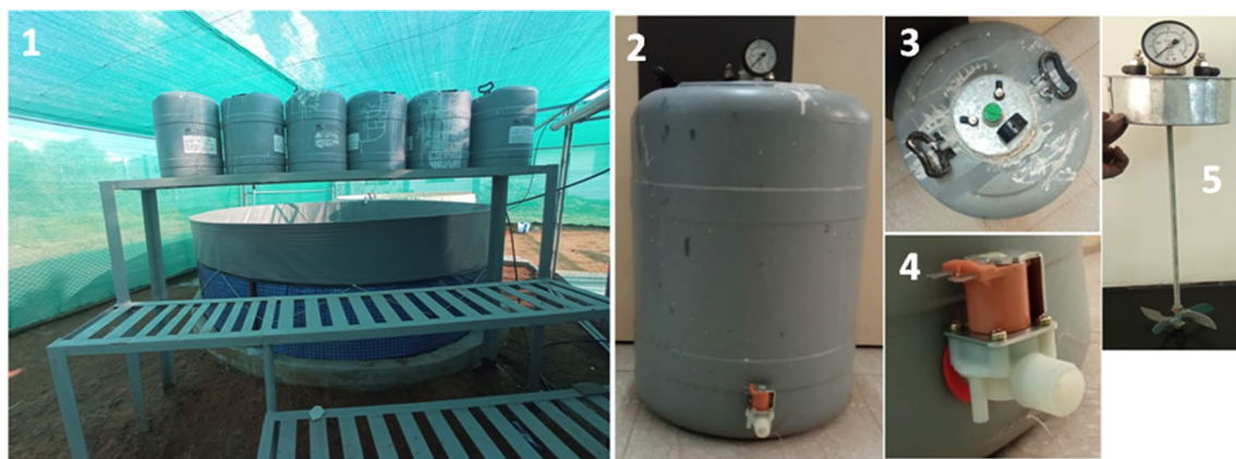
Fig. 3 Top-dressing system with stirring and dispersion units to be used in an aquaculture automation system for Biofloc production of shrimp
