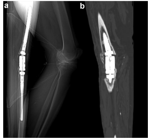
Figure 5. Second reoperation for a patient with mechanical failure. Sagittal views of a computed tomography scan showing significant angulation of the modular knee arthrodesis (a) due to fracture of the proximal diaphyseal connector (b) 6.5 years after implantation.
