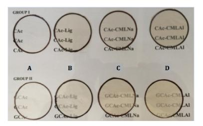
**Figure 1.** Eight membranes of cellulose acetate (CA) produced. The letters A, B, C and D refer to the membranes of groups I and II described in this figure.
