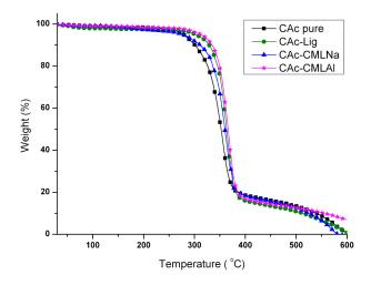
Figure 5. Thermogravimetry (TG) curves for the membranes of group I.
