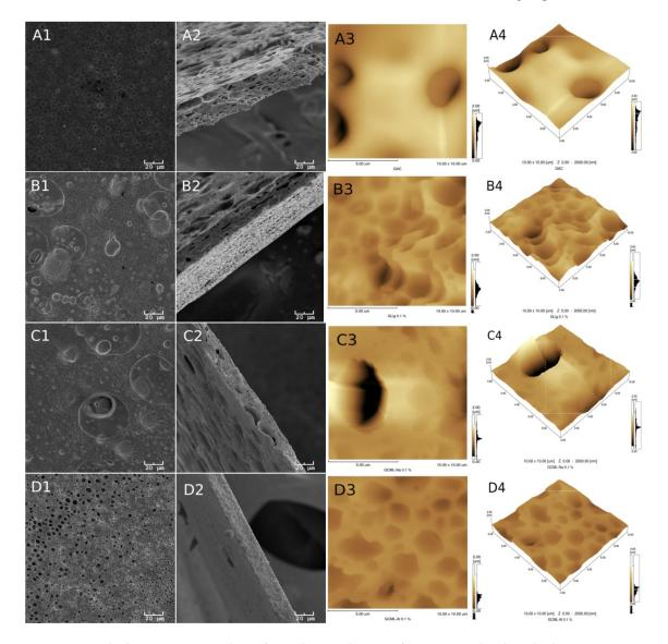
**Figure 3.** The letters A, B, C and D refer to the membranes of groups I and II described in Figure 1. Numbers 1, 2, 3 and 4, in A1 through D4, refer to surface SEMs (1) and fracture (2) of the membranes and the two-dimensional (3) and three-dimensional (4) AFM of the membranes of group II.
