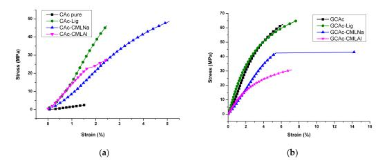
Figure 9. Stress-strain curves for the membranes of groups I (a) and II (b), respectively.
