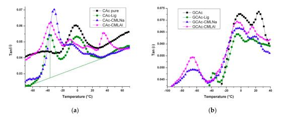
**Figure 8.** Tan  $\delta$  versus temperature for the membranes of groups I (**a**) and II (**b**).
