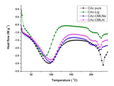
Figure 4. Differential scanning calorimetry (DSC) curves for the membranes of group I.
