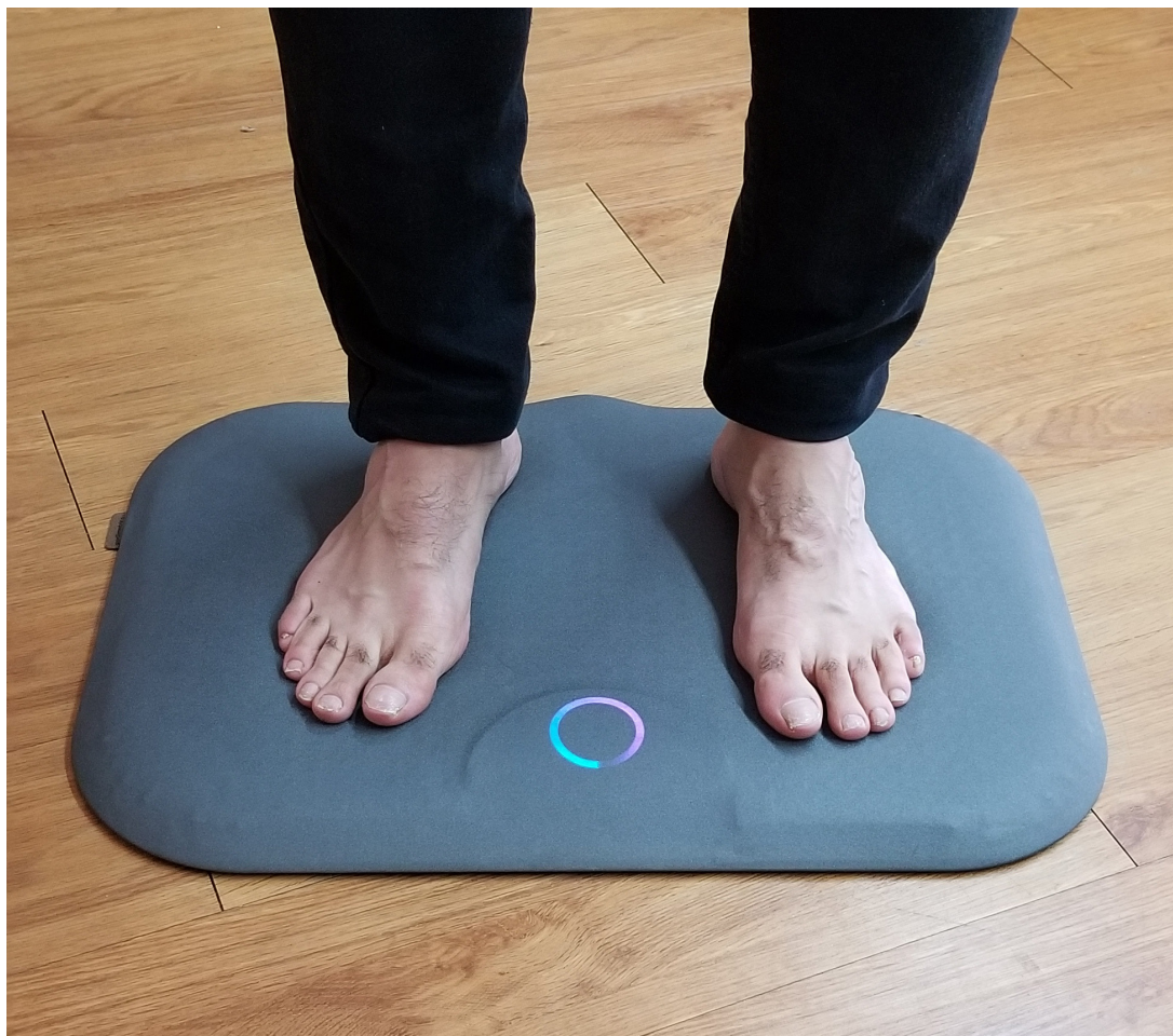
Figure 1 The study device was a telemedicine once-daily foot temperature monitoring mat.
