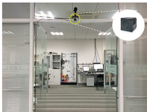
Figure 8. The experimental environment and installation of TOF camera in the laboratory scene.
