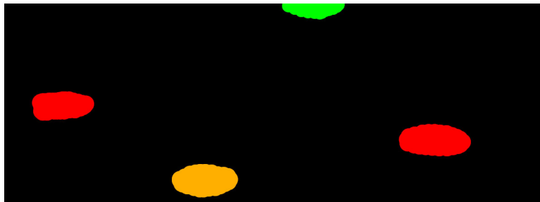
Figure 5. Example of a semantic segmentation label. The red label represents dead knots, the green label stands for live knots, and the dark yellow represents knots with cracks.
