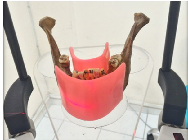
Figure 1. When the CBCT machine became ready to expose, 2-ply modeling waxes were placed buccally and lingually to imitate soft tissues and then the jaws were exposed. (Romexis viewer 3.0.2, Planmeca.)
