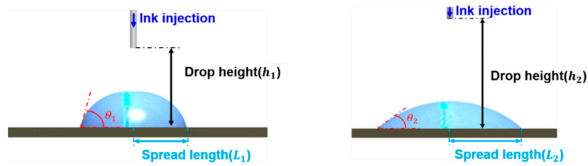
Figure 2. Schematics of the change in the contact angle and coating width by varying the injection height.
