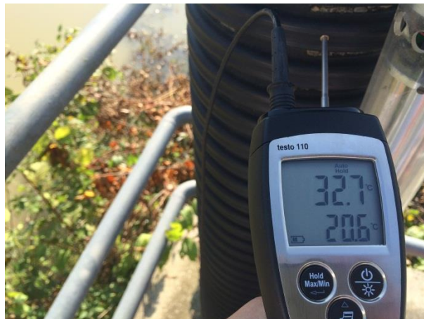
Figure 16. The measured temperatures on the sunny and shady sides of the reference point; the upper value shows the temperature on the sunny side, while the lower value shows the temperature on the shady side.
