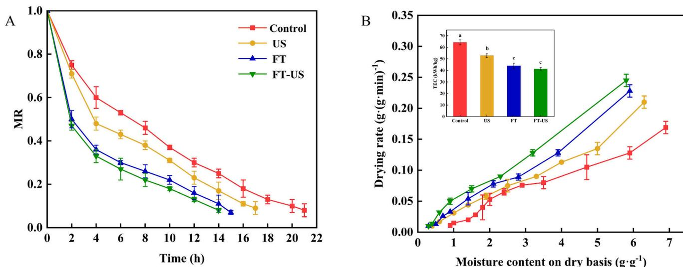
**Fig. 1.** Drying curves of vacuum freeze-drying (VFD) apricot slices with different pretreatments. The relationship between moisture ratio (MR) and drying time (A); Drying rate in relation to moisture content and total energy consumption (B). Different letters in the same row indicated significant differences between pretreatments ( $p < 0.05$ ).
