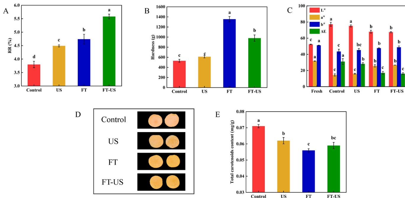
Fig. 4. Rehydration rate of vacuum freeze-drying (VFD) apricot slices with different pretreatments (A); hardness and moisture content (B); color (C); appearance (D) and carotenoid content (E). Different letters in the same row indicated significant differences between pretreatments ( $p < 0.05$ ).
