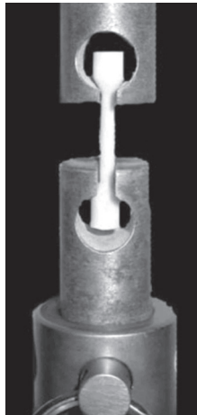
Figure 1- Polyurethane bell-shaped specimen positioned for tension tests
