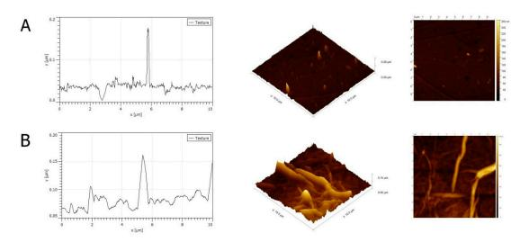
**Figure 2.** Atomic Force Microscopy (AFM) mages and a topography model of the surface of a culture plate (**A**) and graphene oxide nanofilm (**B**).
