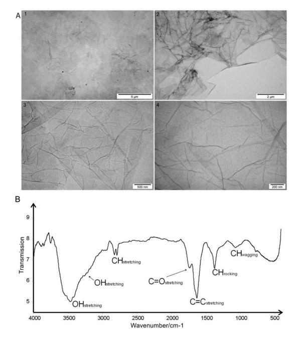
**Figure 1. (A)** Transmission electron microscopic images of graphene oxide flakes at increasing magnification: 1) 5,000, 2) 8,500, 3) 34,000, 4) 70,000; **(B)** Fourier Transform Infrared Spectroscopic spectrum of graphene oxide with the assignment of bands to appropriate vibrations of groups and bonds present in the sample.
