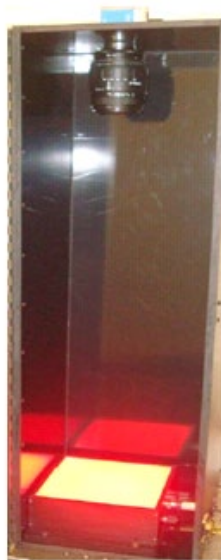
FIG. 2. 2D optical imaging apparatus consisting of a diffuse red light surface and a lens-coupled CCD. Excess area on the light surface was masked using black construction paper to improve the dynamic range of the system.
