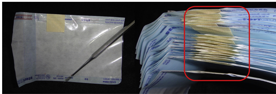
Figure 2. Pouches from a positive control group showing a spatula separating the seal on the side of the pouch. The circled area shows the separated seal.
