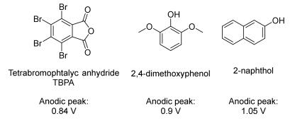
**Figure 6.** Oxidation potential of TBPA, 2,6-dimethylphenol, 2-naphthol. CV conditions: 0.1 mol/L LiClO<sub>4</sub>/CH<sub>3</sub>CN; Pt disk w. e.; Ag wire c. e.; Ag/AgNO<sub>3</sub> 0.1 mol/L in CH<sub>3</sub>CN ref. e.
