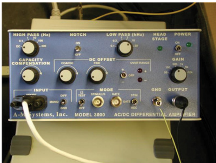
Figure 14. "Test toggle" is in the bottom row to test electrode resistance. The "coarse" knob is also found under DC offset which should be turned counter clock wise. Gain is set to 50, which amplifies signals by a factor of fifty. The ground wire from the head stage is placed in the "GND" pin jack opening.
