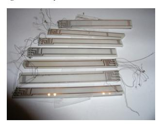
**Figure 11.** Delay lines for SAW vibration sensor.
