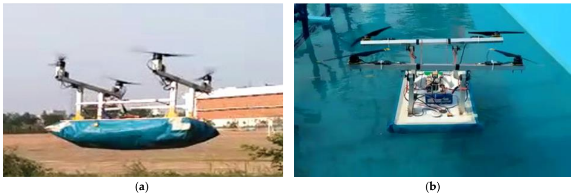
Figure 19. Field testing of amphibious UAV: (a) Amphibious UAV (airborne); (b) Amphibious UAV (gliding above water).
