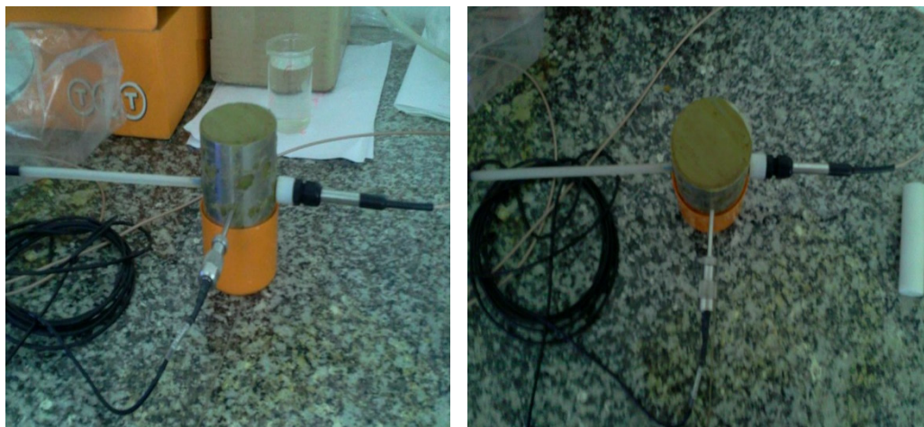
Figure 5. A sample of silty sand with inserted sensors (Laboratory of the Department of Geotechnics, WULS-SGGW).
