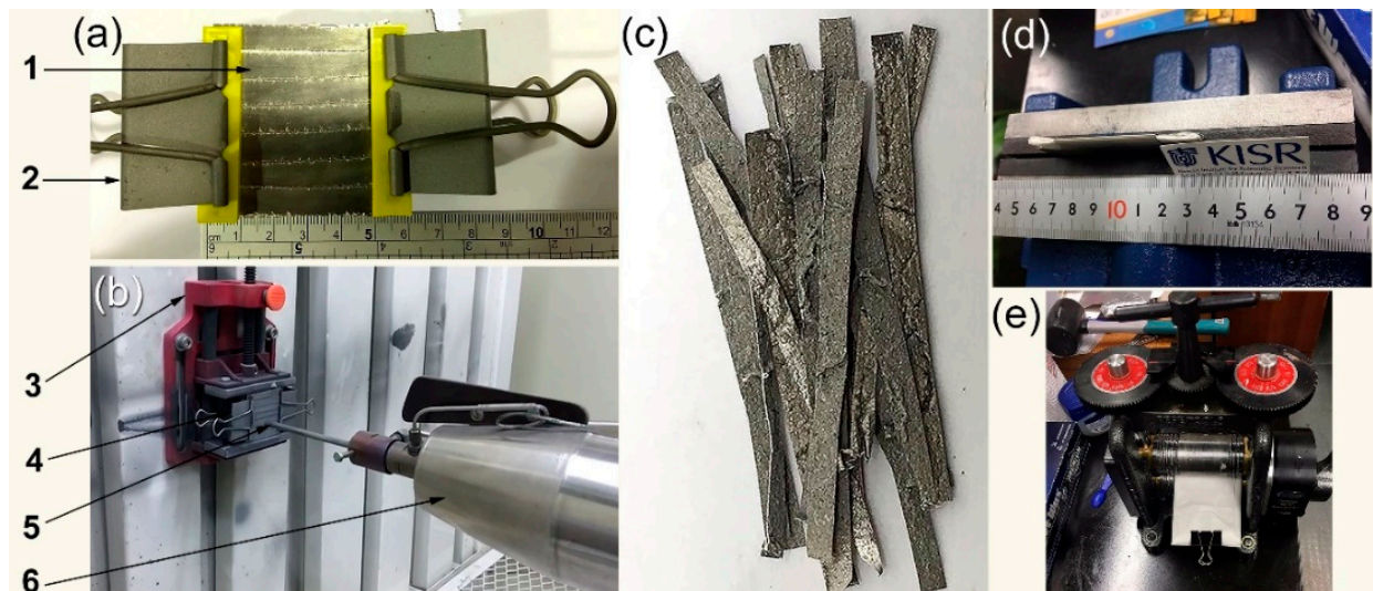
Figure 3. (a) The cold-rolled Mg ribbons (1) were placed and fixed on stainless steel plate by clips (2); (b) two-movable jaws (3) were used to fix the ribbons that was aligned perpendicular (5) to the cold spray (CS) gun nozzle (6). In the image above (c), the Mg-ribbons have been coated three times with Ni powders. To ensure straightening, the uncoated Mg-strips were wrapped in balance papers and put in a two-jaw style vise for 16 h (d), and then CR for 10 times (e).
